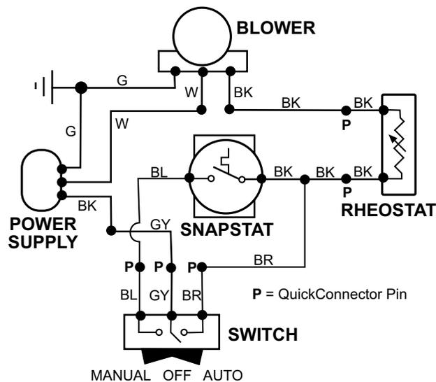
Figure 37. Blower Wiring Diagram
