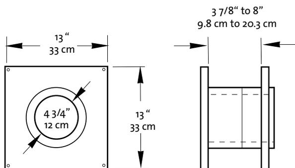
Figure 2. Approved Wall Pass-Through, Simpson Dura-Vent Wall thimble #3143.
