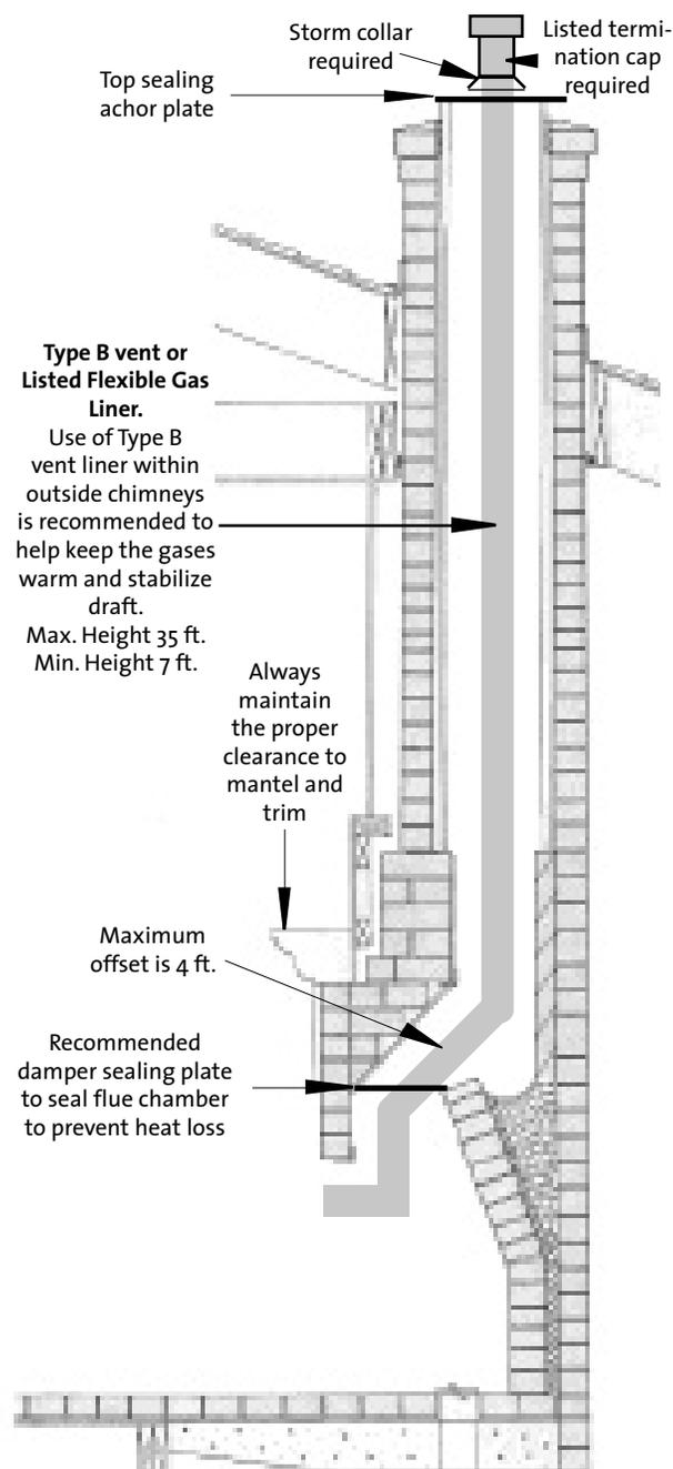
**WARNING: FAILURE TO POSITION THE PARTS IN ACCORDANCE WITH THIS DIAGRAM OR FAILURE TO USE ONLY PARTS SPECIFICALLY APPROVED WITH THIS APPLIANCE MAY RESULT IN PROPERTY DAMAGE OR PERSONAL INJURY.**
