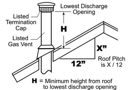
When vent is less than 8 feet from wall, vent termination must be minimum 2 feet above wall.
