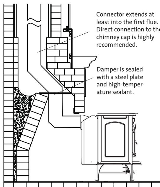
Figure 7. Hearthmount Installation.
