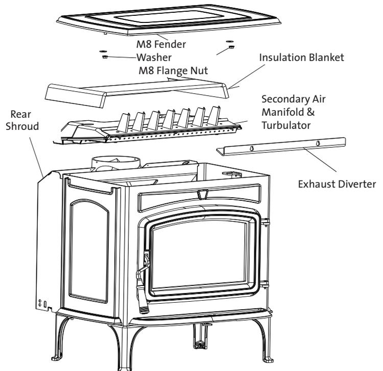
Figure 26. Overview of secondary air manifold removal
