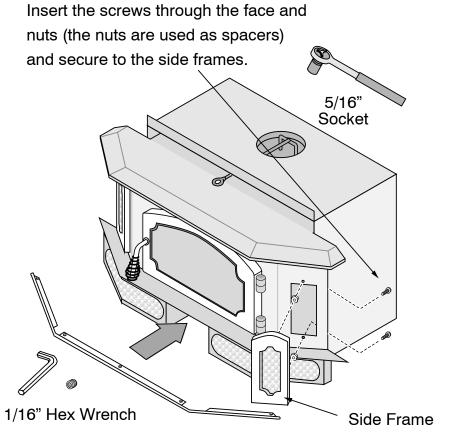
Slide the ashlip trim into place then tighten the five set screws on the bottom of the ashlip to secure.
