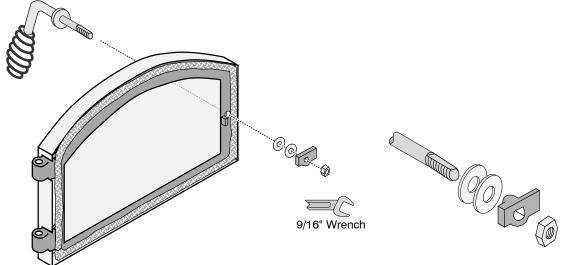
6. Replace the door on the hinges and latch the door.
