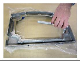
3. Place the door retainer into the door shell as shown below.
