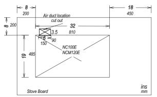
LOCATION AND DIMENSIONS OF AIR INTAKE DUCT HOLE AND FLOOR PROTECTOR AS SEEN FROM TOP
