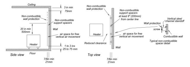
TYPICAL SIDE-WALL PROTECTION FOR CLEARANCE REDUCTION OF 50%
