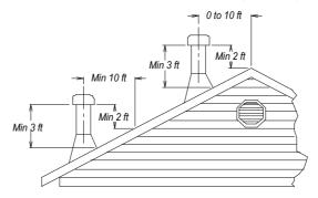
BASIC RULE FOR CHIMNEY TERMINATION HEIGHTS ABOVE ROOF
