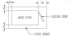
**WARNING:** Install on durable non-combustible and non-heat conducting pad, equivalent to asbestos mill-board of at least 3/8" (10 mm) minimum thickness, which extends at least 8" (205 mm) from the unit on all sides, and 18" (455 mm) from the firedoor end. Alternatively install in accordance with provisions of NFPA 211 (USA) or CAN/CSA-B365 (Canada). Do not obstruct the space beneath the stove.
