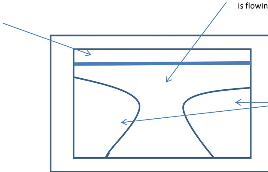
Stain areas; size is function of air velocity. When air velocity is low air wash does not reach the outer edges of glass
