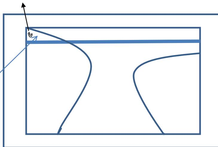
Stain pattern (represents fuel) enters the manifold; oxygen allows combustion and some type of vortex / localized pressure is created. Gases forced out through gasket most likely due to fuel combustion and expansion in the manifold
