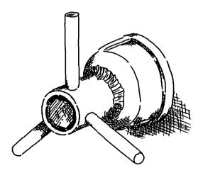
Bob saw a small scale model of a draft cap made out of bolts, pipe and a cut up pipe cap.
