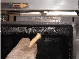
Using a 5/16 nut driver, remove the two screws holding the air spreader bar from the inside top of the door frame (Photo 5).
