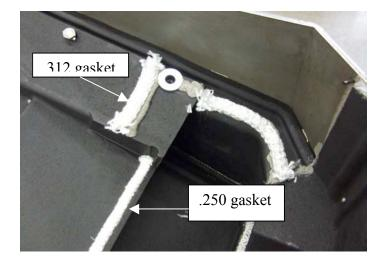
15. Lay the catalyst top upside down on your workbench. Lay a line of gasket glue in the catalyst gasket track and put .250" gasket in the track with and extra 2" of gasket on each end. **NOTE: It is helpful to use a few strips of masking tape to hold the gasket to the glue. Allow the glue to set for 30 minutes before turning the catalyst top over.**
