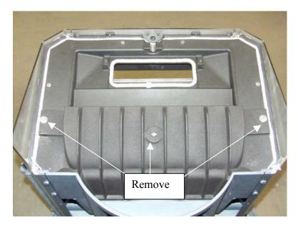
9. Remove the four hex head bolts that hold the lower catalytic combustor plate in place. There are two bolts along the front side and one on the left and right. Remove the plate.
