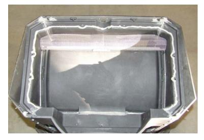
11. Lower a catalyst base/bypass plate (P-325) into place on the stove cement as shown below and secure with (4) <sup>1</sup>/<sub>4</sub>-20 x <sup>3</sup>/<sub>4</sub> HHCS in the front 4 bolt holes, loosely for now.
