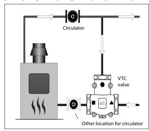
The VTC valve, when placed on the return side will open when the minimum return temperature of the element is reached. When the fluid temperature reaches 18°F (10°C) higher than the element's temperature, the return port from the system will be fully open.
