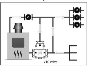
Where a high mass non condensing heat source is matched with a large low temperature system, a situation could occur where the heat source is unable to keep up with the rate of demand from the system. The use of the thermic valve provides the opportunity for the heat source to catch-up.
