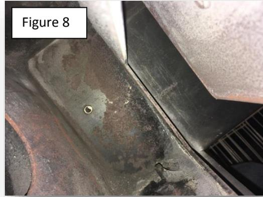
Her is a view from the inside of the smoke chamber in fig 8 you can see the chrome intake of the pressure switch in a Sabrina it is located on the right hand side wall you need to make sure to clean this inlet properly or you will end up whit default start alarm **on a P96x.. it's on the rear wall**
