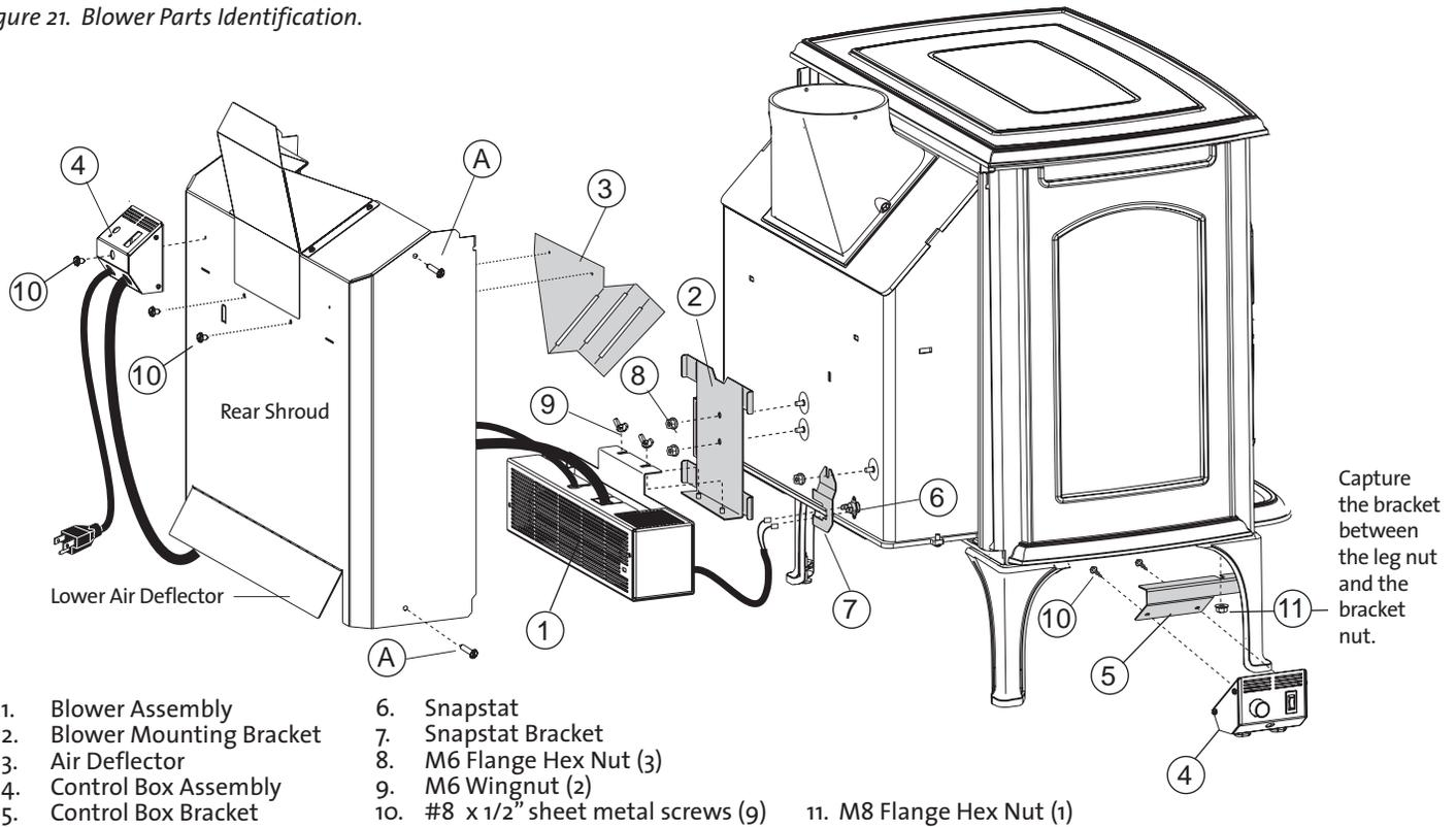
7. Bend back the Lower Air Deflector panel on the rear shroud. Reinstall the shroud by reversing the procedure in Step 1. Engage the shroud with the upper hex nuts on the back of the stove and then reinstall the socket head screws at the bottom of each side.
