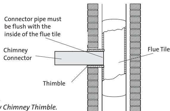
Figure 6. Masonry Chimney Thimble.
