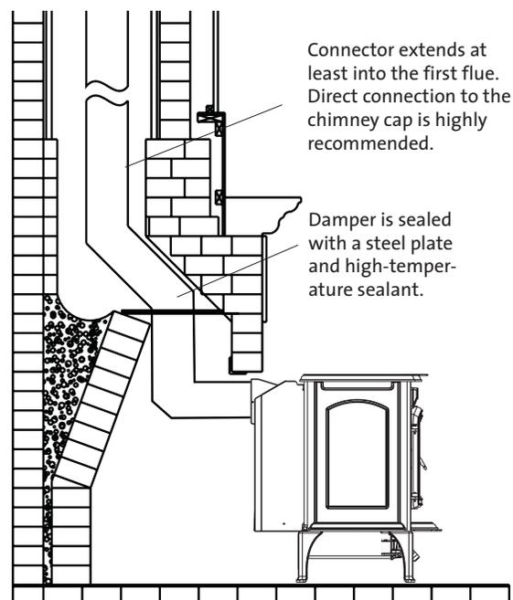
Figure 7. Hearthmount Installation.
