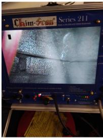
The flue tile is not sealed at the top of the smoke chamber. This can allow the byproducts of combustion to go behind the flue tiles and may migrate to areas of the chimney and home not meant to contain them. The potential hazard exists that combustible residue could built up where it cannot be maintained and allow the possibility of a structure fire. This defect could also allow carbon monoxide the enter the home. 2016 NFPA 211 11.2.1.13
