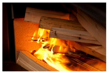
**6 Minutes -** Igniter shuts down and blower continues to push air acting as a bellow to fan the fire.
