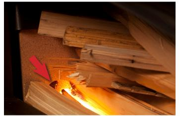
**30 Seconds -** Hot surface igniter blows 1400 degree heated air into firebox igniting the wood.
