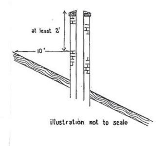
The chimney should terminate at least three feet higher than the roof and two feet higher than any portion of the roof within 10 feet of the chimney. In some cases, even though this quideline is followed, downdraft and puffback may occur. Those problems can be cured by the installation of a chimney cap. If poor draft is the problem, the use of a turbine-type chimney cap can improve draft at the same time it helps prevent downdraft problems.
