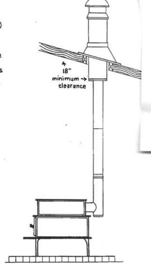
Storepipe clearances should be a minimum of 18 inches from combustibles unless a specific form of protection is employed, to reduce the distance. Do not run storepipe through a window or ceiling. Storepipe should not be run through a wall or partition unless a wall thimble is used and a clearance through the wall
