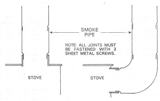
Be sure to maintain at least 18" clearance between the smoke pipe and all combustible materials. Any horizontal runs of stove pipe should have a minimum rise of 1" per running foot of pipe. Horizontal runs should be kept to an absolute minimum. Avoid using more than two elbows. Do not reduce the diameter of the smoke pipe to less than the diameter of the flue collar.
