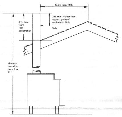
Minimum chimney heights above roof and clearances.
