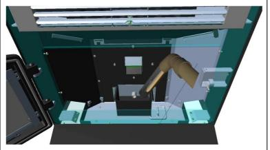
After removing the burn pot vacuum the ash within the burn pot receptacle.
