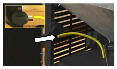
Blow into the tube and ensure that the air passes freely.
