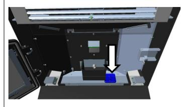
Vacuum the ash at the bottom of the pan and make sure the ash dump plug is in place and tight.
