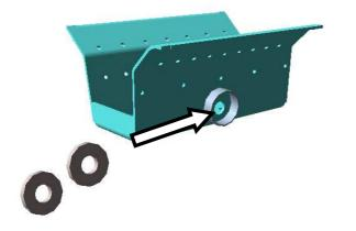
It is important to insert 2 Gaskets into the receptacle behind the burn pot. In the absence of gaskets the stove will not light easily.
