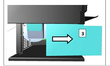
The Access to the exhaust fan is on the left side of the pedestal. Follow these steps To remove the left panel of the pedestal.
