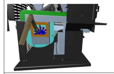
Vacuum the ash and clean the fins of the fan using a small brush.
