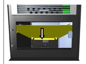
2. Lower the baffle until the tab is behind the burn pot receptacle.
