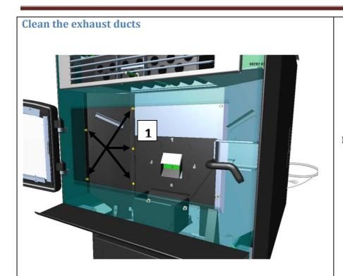
To access the exhaust ducts, remove the wall on the left side of the burn pot.
