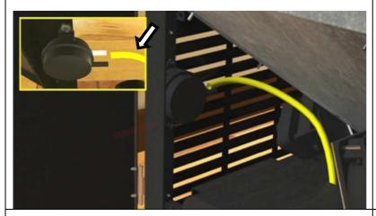
Remove the tube from the pressure sensor.
