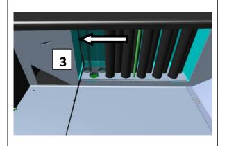
It is difficult to insert the vacuum hose into the openings. Using a ¾ inch hose installed on a vacuum adapter will facilitate access to these tight spaces.
