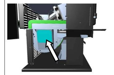
Remove the plate from the exhaust fan by unbolting the 4 bolts.
