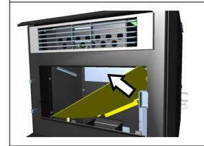
4. Continue rotating the baffle to remove it completely.
