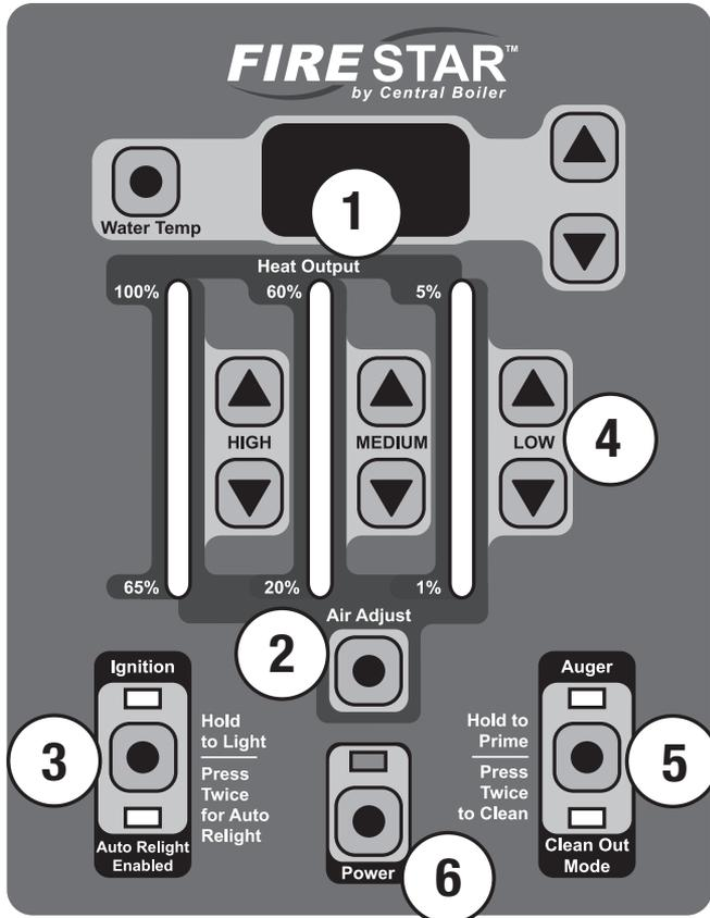
1. During normal operation, the LED display indicates the actual temperature of the system water. Other information will also be displayed on the LED display depending on settings, modes, etc. The **Water Temp** button may be used to display the water temperature setting or, used in conjunction with the up and down buttons, to change the water temperature setting.
