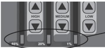
Bottom three LED lights will flash to indicate Cold Burner (see description below)
