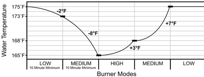
If burner temperature is not high enough the controller will not switch from MEDIUM to HIGH mode.
