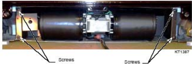
Fig. 3 Remove blower assembly.
