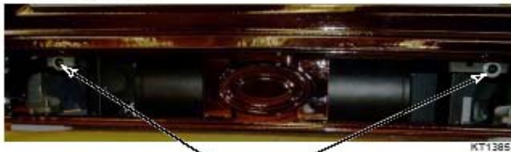
Fig. 1 Remove the two (2) Phillips head screws.
