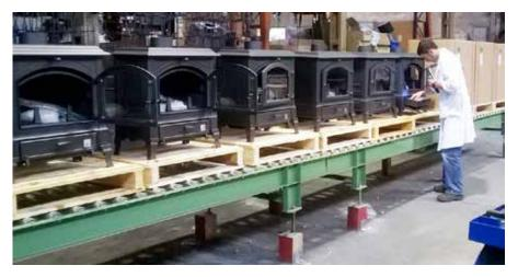
Once the preproduction run has been completed the stoves can go into production in full. The picture above shows the first Harmony 1 multifuel stoves on the quality control line.
