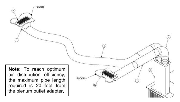
(I) – In regards to part (I) there are three different products you can use for your installation: semi-rigid tubing, galvanized rigid tubes or insulated aluminum tube. In all cases the material must be at least 325°F resistant and must respect the 1" clearance to combustible materials mentioned above.
