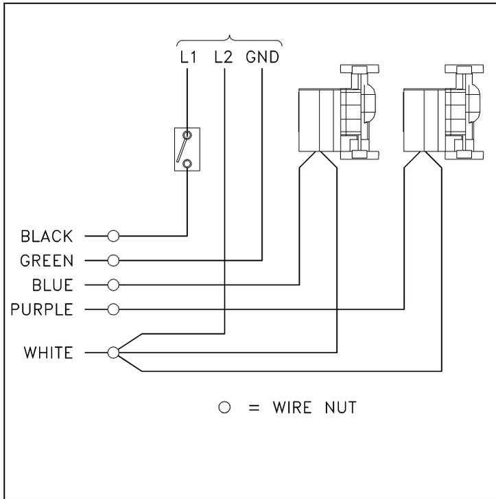
Figure 12-2 Low Voltage Wiring
