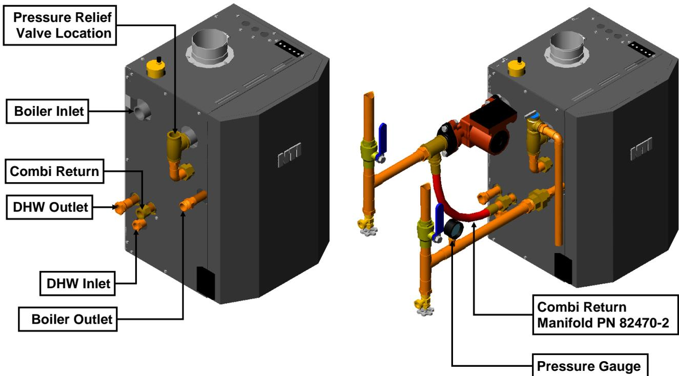
Figure 10-1(c) Near Boiler Piping – Combi (Ti150 Canada)
