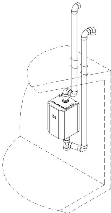
Figure 4-3(b) Concentric Roof Termination
