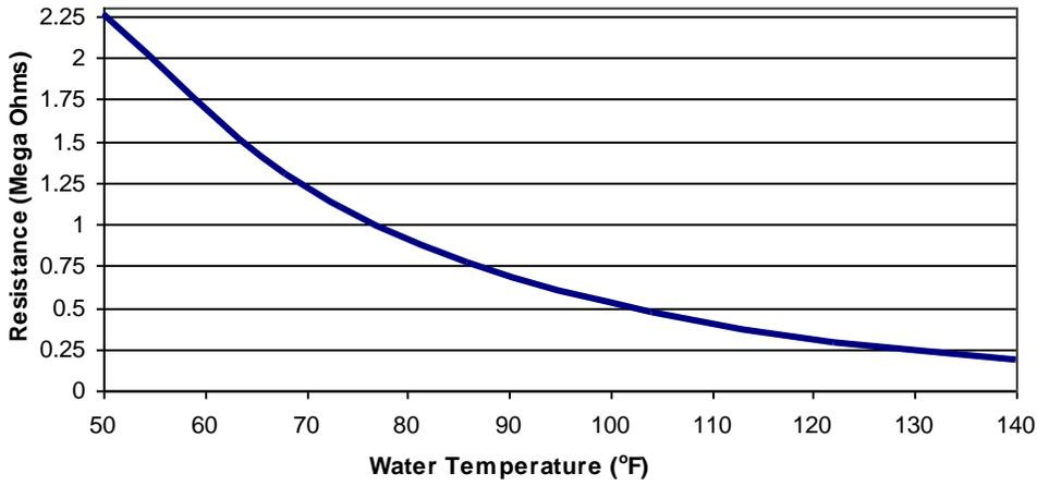
Figure 18-2 Thermistor Resistance Chart – 1 MOhm Water Probe (High Temp.)
