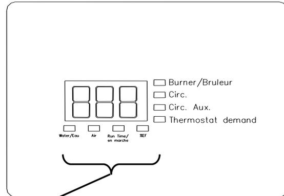
**Water Temp** – When illuminated, indicates that the display is showing boiler water temperature.
