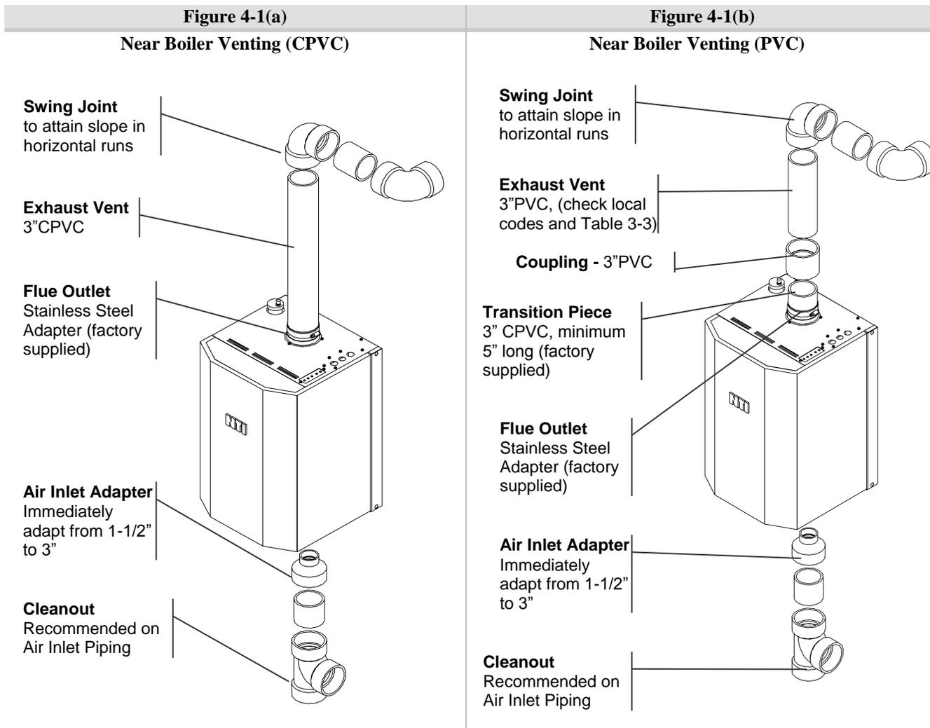
\* **Air-Inlet** - check with applicable local codes for acceptable pipe material.
