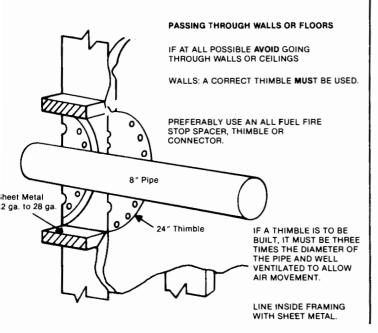
CONNECTING THE STOVE PIPE TO A CHIMNEY, THROUGH A WALL
