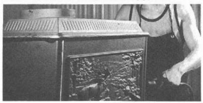
At the next station, the chrome latches and finials are perfectly fitted by a skilled craftsman, and the door liners are inserted.
