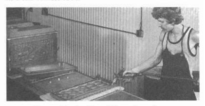
Once the body of the stove is together it is moved along the assembly line to be completely wire brushed and cleaned before being painted. This procedure reduces the possibility of chipping and rough spots. Upland uses 1100°F Thermolux paint on its stoves. The painter carefully inspects each stove he works on before and after the paint is applied.
