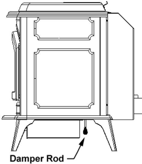
2. Screw damper rod into threaded hole.
