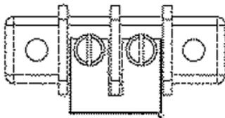
Remove Jumper if Thermostat Is To Be Used
