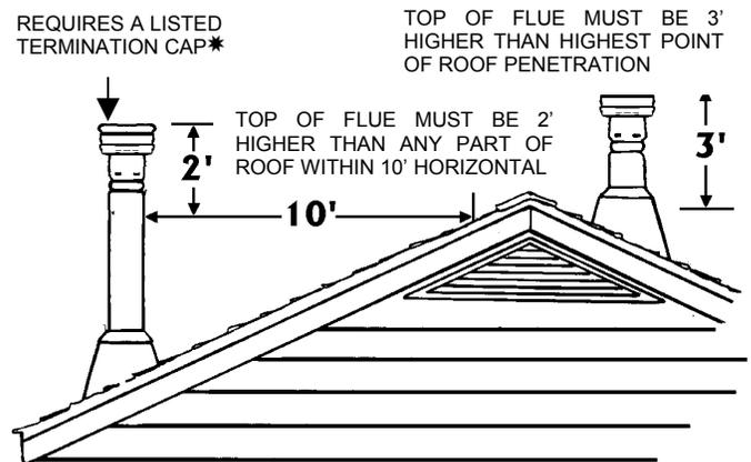
To pass inspection in nearly any jurisdiction, the chimney must meet both safety and exhaust flow requirements. The (3' by 2' by 10' rule applies to both masonry and factory built chimneys.
