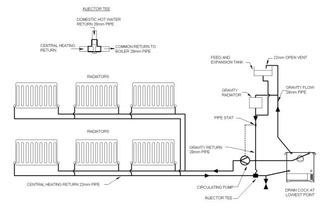
Note: Diagrammatic representation only. Design and calculations for individual systems should always be carried out by a qualified heating engineer.
