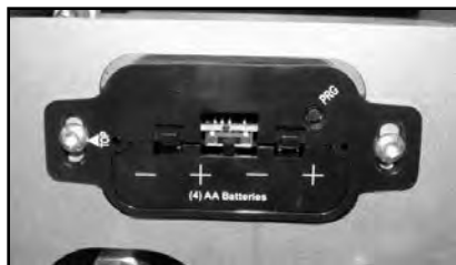
Figure 4. On/Off switch. Position switch in the middle to use the hand-held remote control unit.
