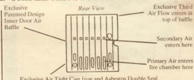
Exclusive Air Tight Cast Iron and Asbestos Double Seal Door makes stove airtight and controls burning.
