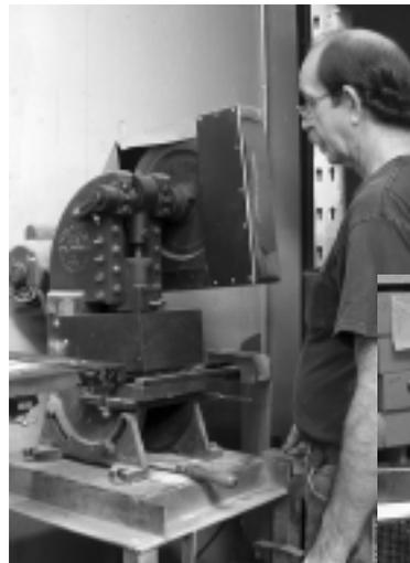
*Roger Parker stamps the Condar brand on the steel of a combustor in the Columbus factory. All Condar combustors are stamped with our brand for customer assurance.*
