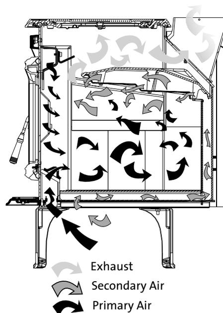
Figure 15. Combustion air paths
