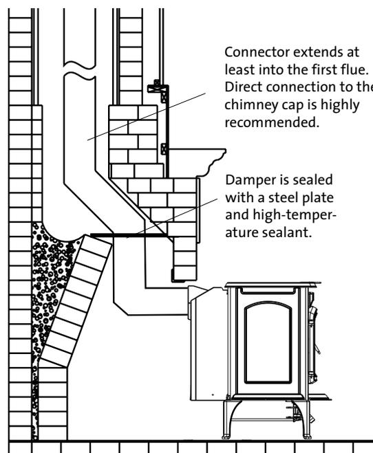
Figure 7. Hearthmount Installation.
