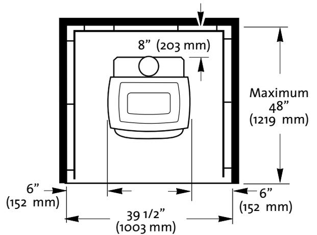
Figure 12. Alcove with Wall Protection.
