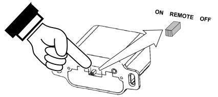
**NOTE**: When the battery holder switch is turned to ON or OFF, the mode settings (Flame Height, Comfort Control) will remain in the same state as before the switch was moved (i.e.: the IFC "remembers" the last setting). If you wish to adjust the mode settings use the transmitter mode button to adjust the settings (see "Mode Controls" on page 12). The thermostat and burner on/off operating functions will not work on the transmitter.
