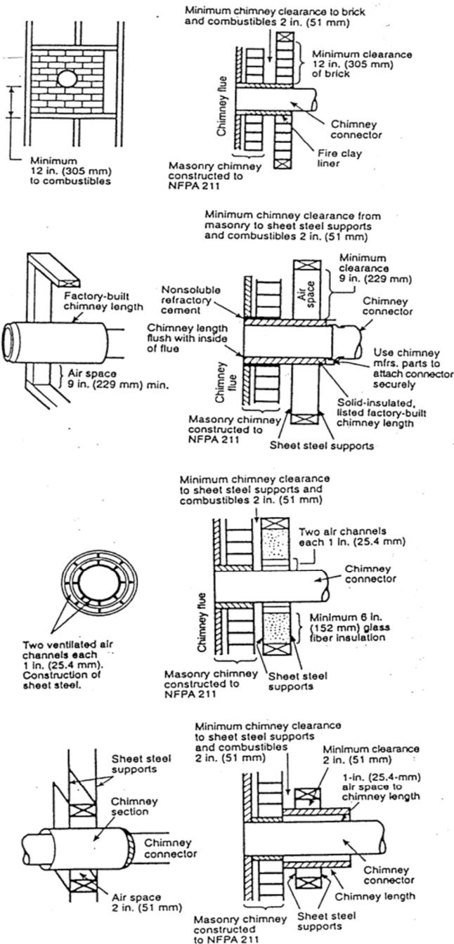
A Minimum 3.5-in thick brick masonry all framed into combustible wall with a minimum of 12-in brick separation from clay liner to combustibles. The fireclay liner shall run from outer surface of brick wall to, but not beyond, the inner surface of chimney flue liner and shall be firmly cemented in place.
