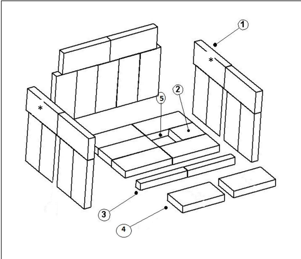
NOTE: The bricks on the sides and rear will need to be installed after delivery
