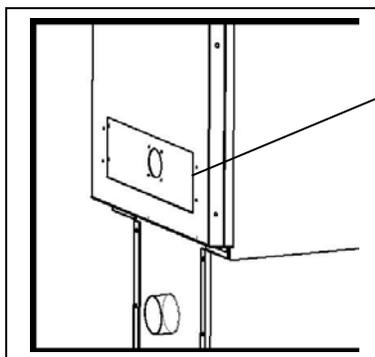
(4) 5/16" head, self-tapping screws (pre-installed in unit).
