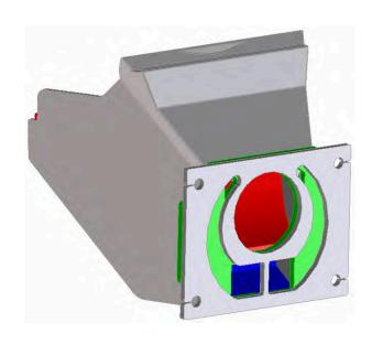
The Accentra Insert and the P-68 have their burnpots designed to accommodate over-fire air. This allows for a more complete burn because of total gas combustion
