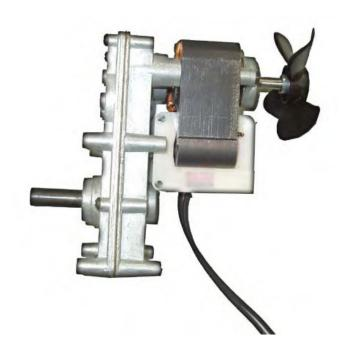
The Advance and Accentra models use a clockwise directional feed motor. This is identified by either two white leads, on older units or black and red leads on the newer ones. It is also a 4 r.p.m. Motor, just turning the opposite direction for the chain drive.
