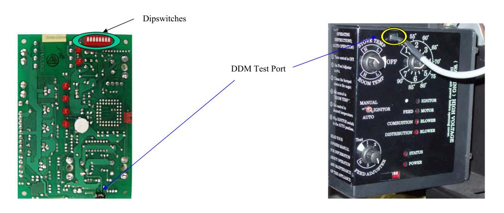
All Harman automatic pellet stoves now use the same circuit board. There is a series of switches on the board, (dipswitches), that are set differently depending on the stove model it is installed onto. Some switches allow for changing things such as ignition feed cycle, or igniter timing. Included on the new circuit board is a test port to attach the DDM, Digital Diagnostic Meter.
