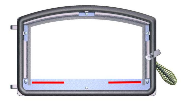
Remove the 4 glass retainers that are secured by (6) phillips head screws.
