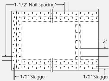
\*When end stiffeners extend through the beam, nail spacing is the same as for flanges, except space nails **1 in. on center** when double end stiffeners are used in beams with three members per flange (cross-section C). When end stiffeners are inserted between flanges, nails may be spaced 3 inches on center.
