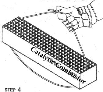
GENTLY PLACE THE COMBUSTOR INTO THE CLEANING SOLUTION.
