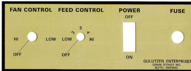
**FEED CONTROL:** This Control is like the Thermostat in your home. The Higher the Setting, the more Grain is fed into the Firepot and the more heat is generated. Over a period of time, you will learn the best and most efficient settings for your particular installation.
