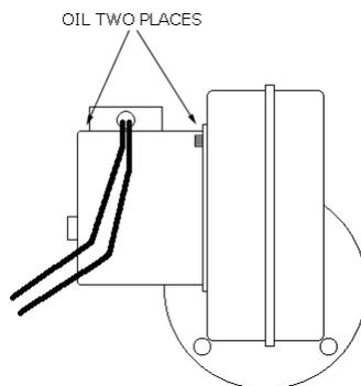
**NOTE:** Both fans have oiling points placed at the bearing ends of the motor.
