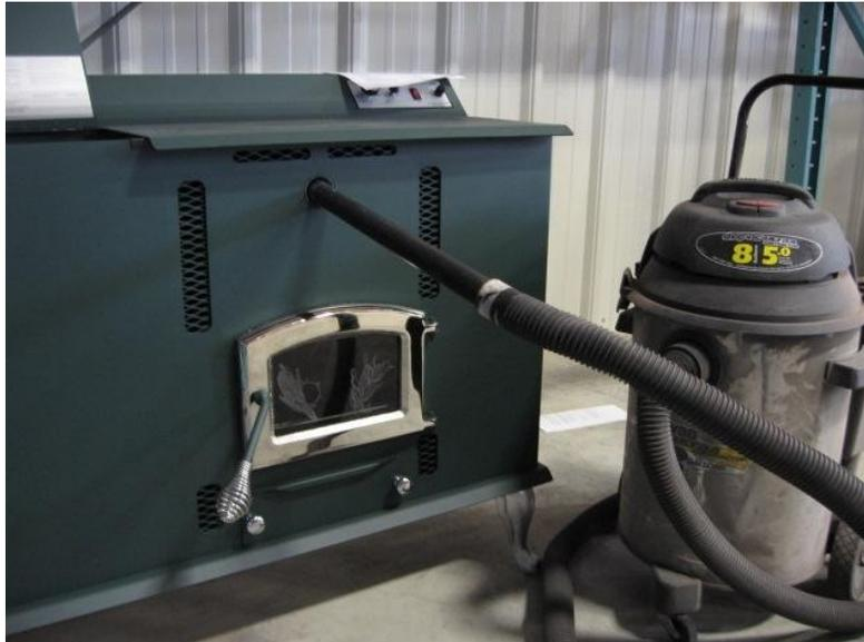
**WITH A SHOP-VAC ON “BLOW”, BLOW OUT THE HEAT EXCHANGER PLATE FOR APPROXIMATELY 1-2 MINUTES**
