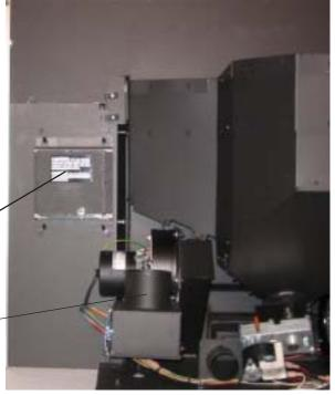
Looking at the back of the stove, you can clearly see the control board hanging on the side flange panel
