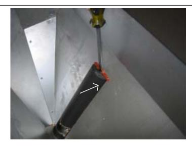
During reinstallation, insert a center punch into the end of the auger shaft and tap on the punch rather than the shaft. Tapping directly on the auger shaft with a hammer will deform the shaft, and not allow the auger motor to be reinstalled.
