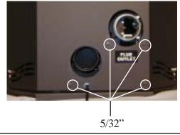
Loosen the two 5/32" allen head screws on both sides of the unit. The back can now be slid back and lifted straight up and off the unit.
