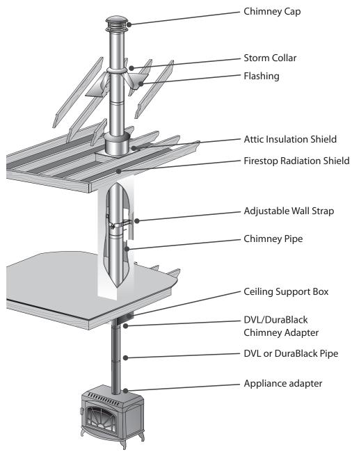
Designed for appliances that are tested and listed for use with a 2100° F HT chimney system.
