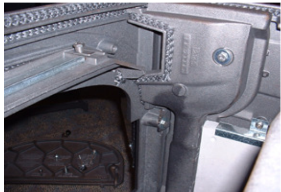
FIG. 13 Main Manifold Removed
