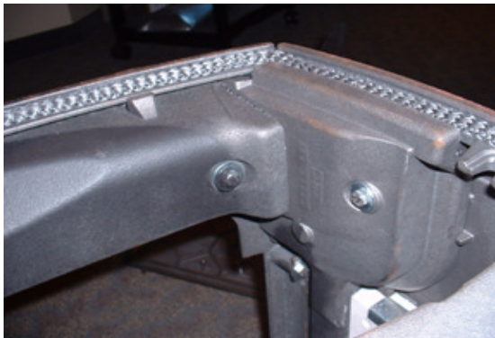
FIG. 12 Air Wash Manifold Left Bolt
