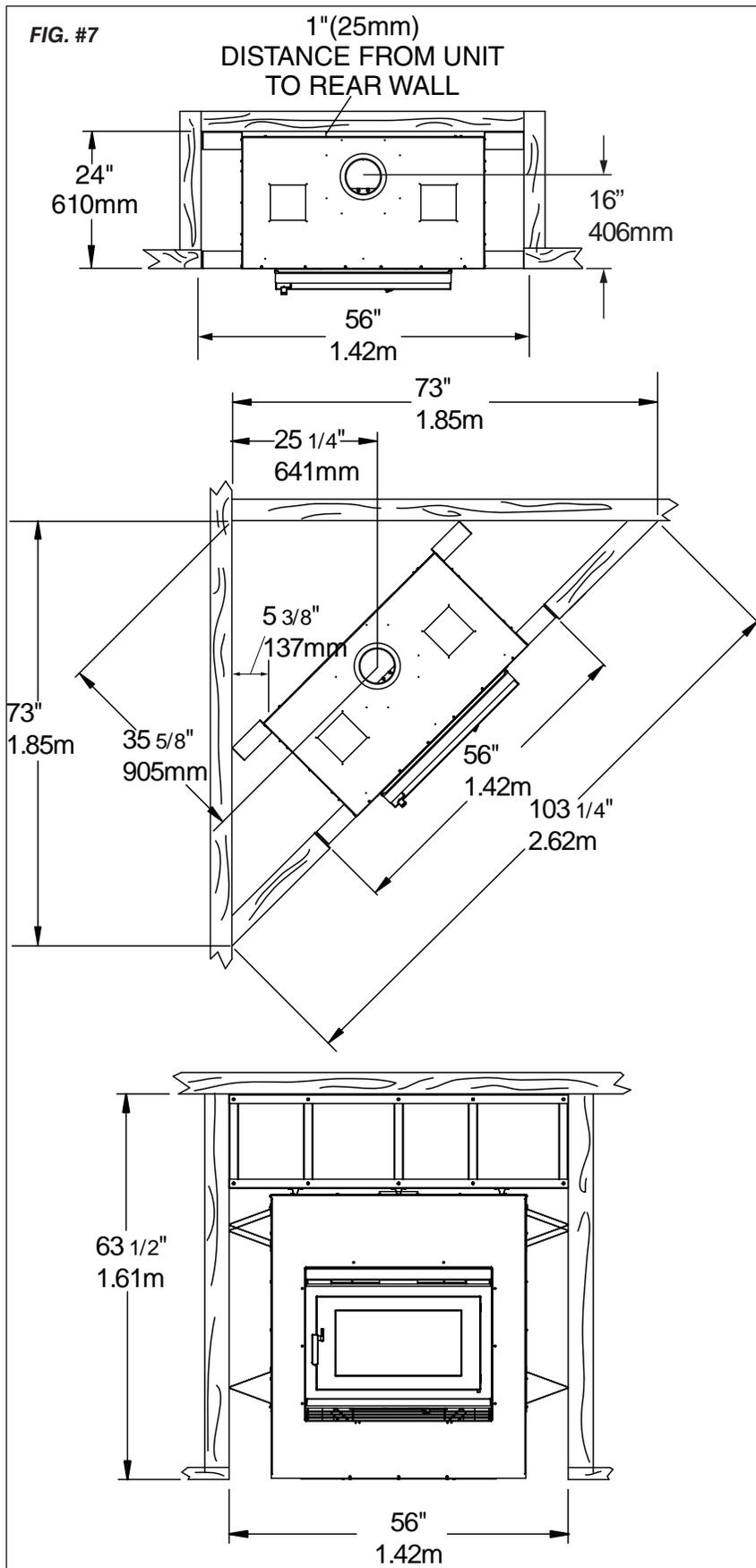
**NOTE: THE FRAMING DIMENSIONS AROUND THE FIREPLACE INCLUDE THE INNER DRYWALL BOARD.**
