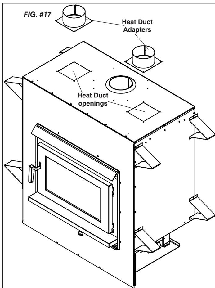
2. Insert a remote heat flap box in the opening/s that you are attaching a kit to. Attach the heat duct adapter/s with the screws provided in the WODC.RHKA (Fig. #17).
