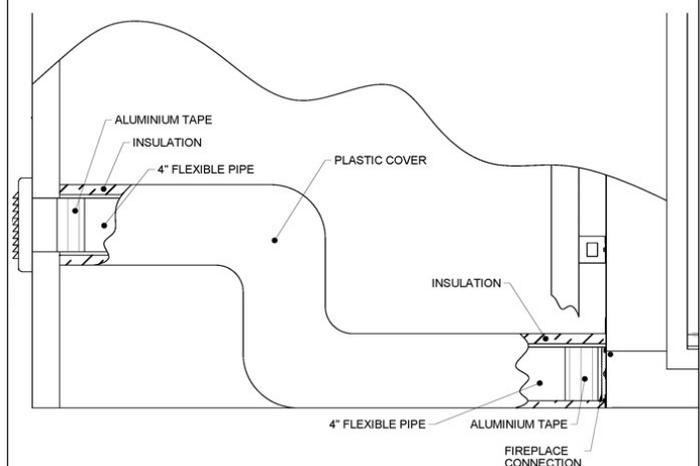
**WARNING: THE COMBUSTION AIR INLET MUST BE AT LEAST 5ft BELOW CHIMNEY OUTLET AND MUST NEVER TERMINATE IN ATTIC SPACES OR GARAGES.**
