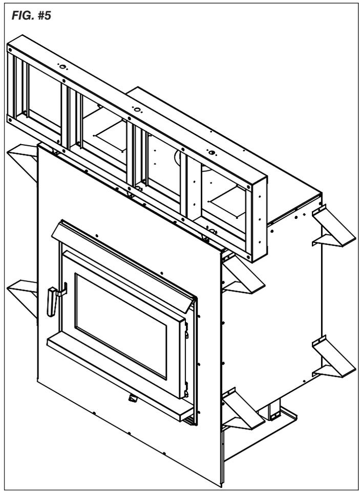
The fireplace must not be in contact with any insulation or loose filling material. Cover the insulation with drywall/ sheetrock panels around the fireplace.
