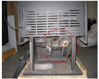
Between the two venting assemblys is the motor.
