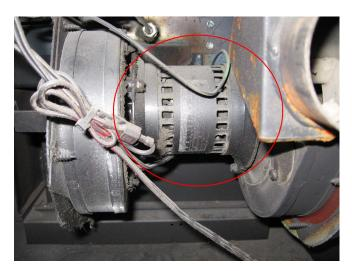
3- Usually the problematic models are the A.O Smith fans, they have little black fins that cool down the motor and these little fins can move and end up hitting the venting assembly, causing the noise.
