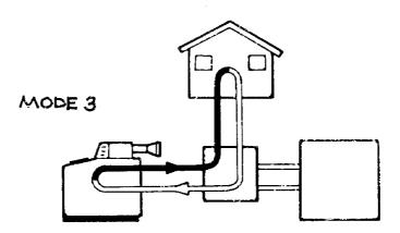
A backup furnace can provide heat when the Jetstream is not being fired and the storage is cold.
