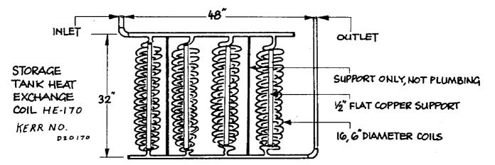
Coil rating should be 170,000 BTU/h at 40 F temperature differential and 10 gallons per minute(U.S.). A typical coil with 1 1/4" connections, as illustrated above would consist of 4 coils of 1/2" finned copper 16 turns in 32 inches. NOTE - This type of coil is recommended to ensure good heat transfer when taking heat from storage.
