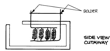
Now lower the Heat Exchanger until the crosspiece supports it. The Heat Exchanger should NOT be resting on the tank bottom.
