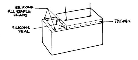
Place the small part of the top (hatch cover) on.
