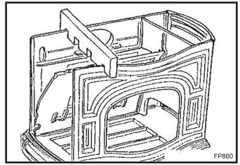
Fig. 3 Wooden bridge in place.
