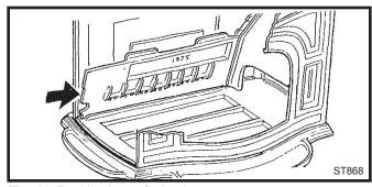
Fig. 10 Position lower fireback.
