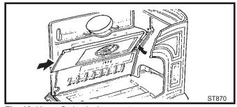
Fig. 12 Upper fireback placement.
