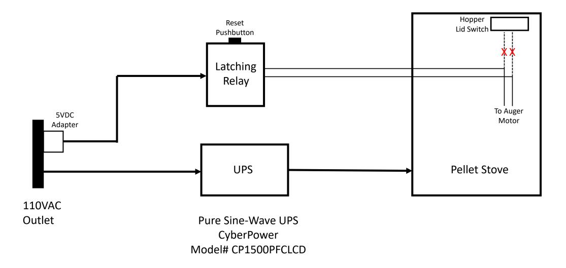
Auto Shutdown of Pellet Stove During 110VAC Power Failure
