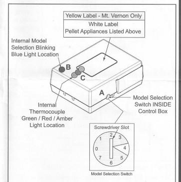
Model Selection Switch is shown with the cover off. Insert flat head screwdriver and rotate cover to expose desired setting number. Refer to table on reverse side for setting information.
