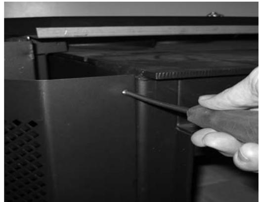
7) Remove wing screws on each side of the Bay top and set Bay top aside to prevent damage. (Fig. #12).
