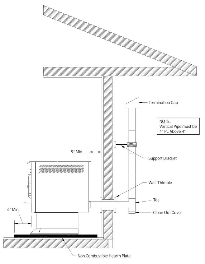
The Hearth Pad is not required under the unit if the floor is noncombustible but is required 6 inches (152mm) beyond the front of the unit and 6 inches (152mm) beyond each side of the door if the floor is a combustble floor. wood flooring, carpet, linoleum, etc.
