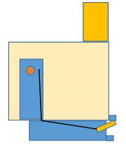
Shim the inlet so damper opens fully Old defiant damper was external opening New VC Flexburn damper opens in
